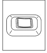
Your vehicle may have this feature. The driver's and passenger's seatback lumbar support can be adjusted by moving the control located on the outboard side of the seat cushions.
